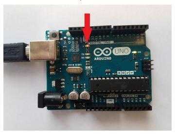
The built-in LED is connected to <u>port B, channel 5</u>, which in turn is connected to digital pin 13 on the Arduino Uno.
